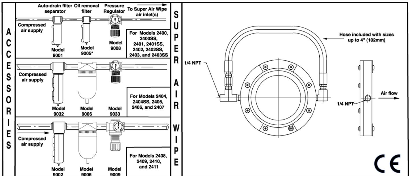
\* Use Model 9006 Oil Removal Filter for Super Air Wipes that are 3" (76mm) and larger
