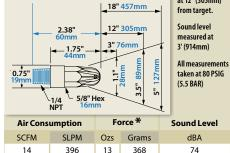
Dimensions and Airflow Pattern \*Force measured
