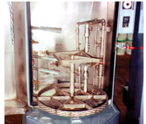
(3) Model 2012 12" (305mm) Standard Air Knives perform the drying cycle in this parts washer.
