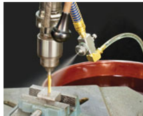
A Model SR1010SS is used to supply a cooling mist for a drilling operation.
