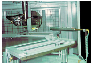
A Model 8212 12" (305mm) Gen4 Standard Ion Air Knife System cleans metal frames prior to powder coating.
