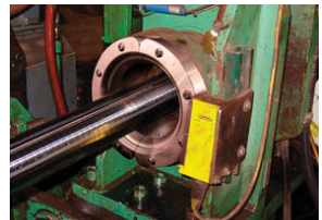
A Model 2404 4" (102mm) Super Air Wipe cleans a steel rod after processing.
