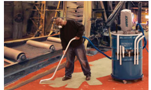
110 Gallon Heavy Duty Dry Vac provides maximum capacity cleanup for a large, dusty walnut shell blasting application.
