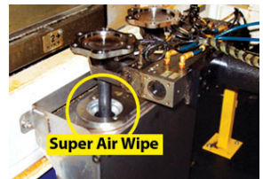
The flanged end of an axle is lifted through a Super Air Wipe to blow off chips after machining.
