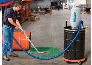
The Heavy Duty Dry Vac cleans up a spill of tumbling media.
