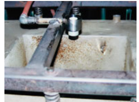
A Model 121021 1-1/4" (32mm) High Temperature Air Amplifier directs hot air to a rotational mold cavity for uniform wall thickness of the plastic part.
