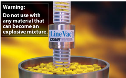
A 316 Stainless Steel Line Vac is used by a pharmaceutical company to convey pills and tablets to a packaging station.
