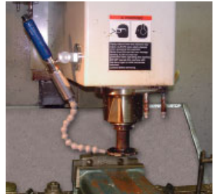
The Adjustable Spot Cooler replaces fluid coolant and eliminates hours of cleanup on a cast iron machining operation.
