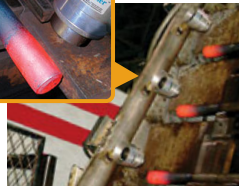
Model 6042 2” (51mm) Adjustable Air Amplifiers with swivel fittings cool inductively heated axles prior to installing the hubs.
