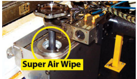
The Super Air Wipe Kit includes a stainless steel shim set, filter separator and pressure regulator (with coupler).
