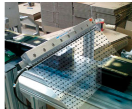
The Model 112118 18" (457mm) Gen4 Super Ion Air Knife System eliminates dust from body care products prior to sealing the boxes in cellophane.
