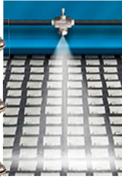
A Model AF1030SS is used to spray an anti-corrosion coating on stamped steel parts as they travel on a conveyor.
