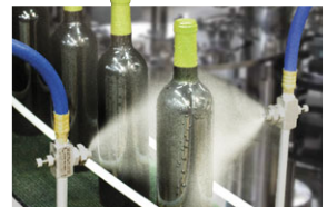
(2) Model EB103055 atomizing nozzles are used to give a final sanitary rinse prior to labeling wine bottles.
