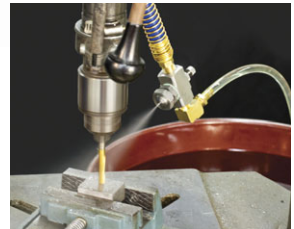
A Model SR101055 is used to supply a cooling mist for a drilling operation.
