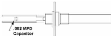
The Model 4519 Capacitor prevents thermostat contact bounce and solenoid chatter due to small switching loads. Wire this capacitor in parallel (across the leads) of the Model 9017 Thermostat. The capacitor is rated .002 Microfarad, 250 VAC, 50/60 Hz.
