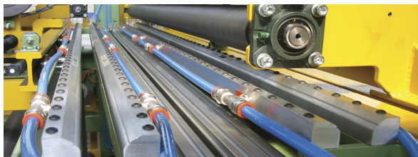
A series of Full-Flow Air Knives "float" layers of plastic film in the confined space of the machine.
