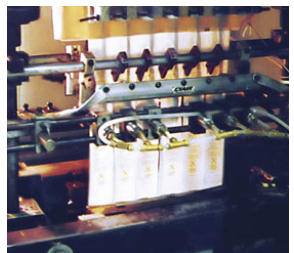
A Model 2012 12" (305mm) Standard Air Knife opens mustard packets prior to fill.
