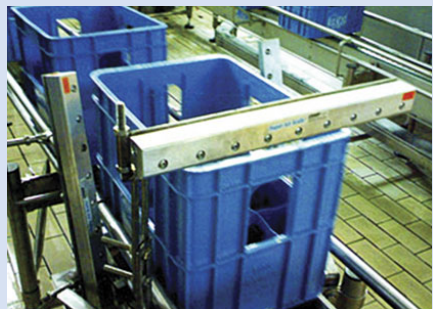
Three Model 110018 18" (457mm) Super Air Knives completely surround and blowoff crates so they can be loaded immediately.
