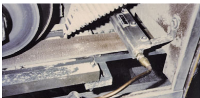
A Model 2006 6" (152mm) Standard Air Knife blows powder loose from a belt so it can be vacuumed away.
