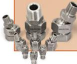
EXAIR's Swivel Fittings make it easy to adjust the aim of the Air Nozzles and Jets. Correct placement of the blowing angle can help optimize performance, reduce noise levels and improve efficiency. Swivel Fittings permit a movement of 25 degrees from the center axis for a total movement of 50 degrees. Type 303 or 316 Stainless Steel.
