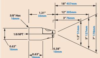
The Model HP1136SS Shim Set for the 1" High Power Flat Super Air Nozzle includes a .020" (0.51mm) and .030" (0.76mm) thick shim. A .025" (0.64mm) shim is installed.
