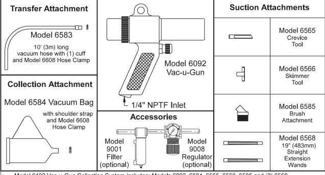
Model 6192 Vac-u-Gun Collection System includes: Models 6092, 6584, 6565, 6566, 6585 and (2) 6568 Model 6292 Vac-u-Gun Transfer System includes: Models 6092, 6583, 6565, 6566, 6585 and (2) 6568 Model 6392 Vac-u-Gun All Purpose System includes: Models 6092, 6583, 6584, 6565, 6566, 6585 and (2) 6568
